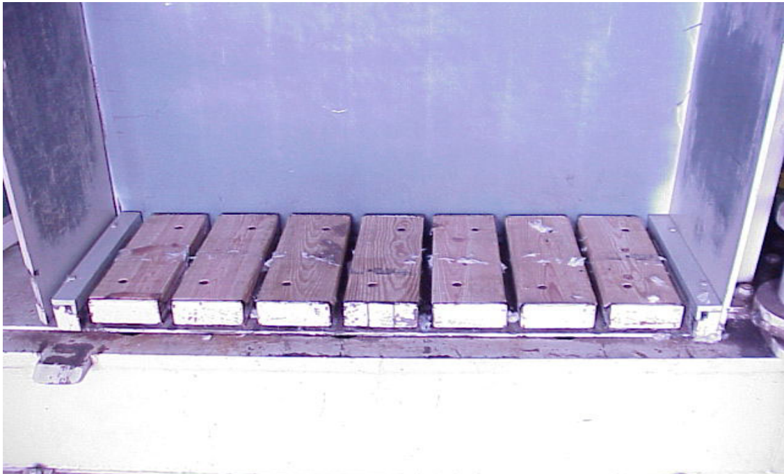
Figure 2. Wooden inserts installed on the standard platen. Similar ones were used on the top platen for all treatments.
