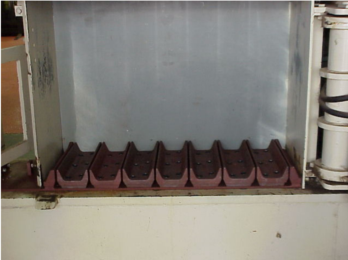
Figure 3. Cast steel platen used on the bottom platen.
