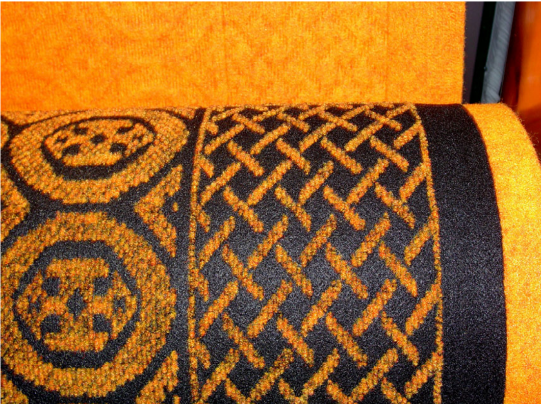
Figure 3. Fehrer end-bordered nonwoven carpet.
