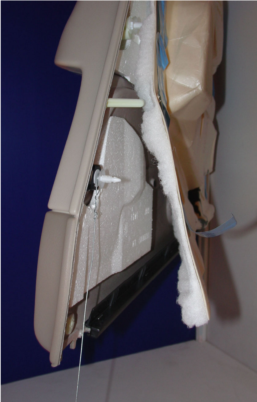
Figure 4. Struto vertical laid nonwovens.
