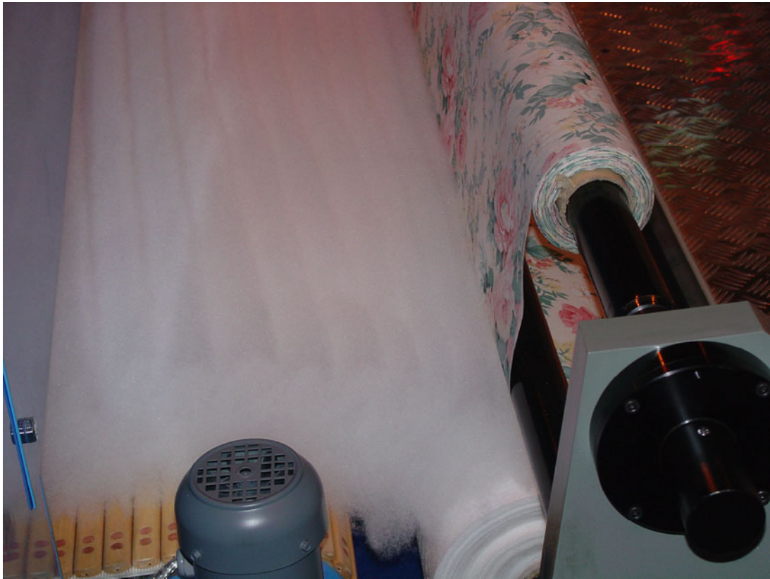
Figure 5. Mazios continuous bat forming/quilting.
