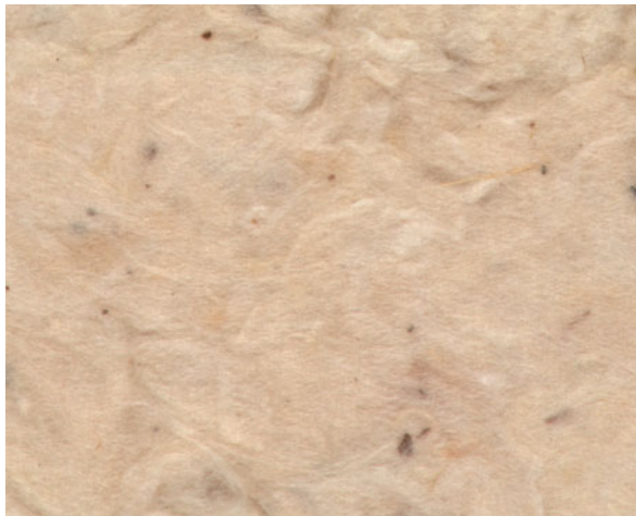
Figure 3. Cotton image and the segmented binary image of MQ356 Lot 5A – Rep 9 (minimum trash content).
