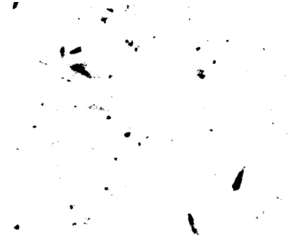
Figure 6. Cotton image and the segmented binary image of MQ356 Lot 13A – Rep 1 (maximum trash content).
