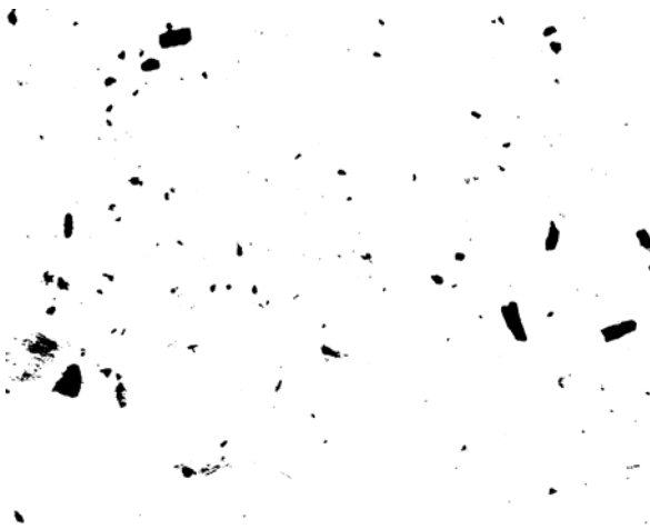
Figure 7. Cotton image and the segmented binary image of MQ356 Lot 13A – Rep 10 (maximum trash content).
