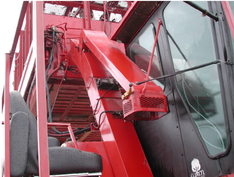
Figure 5. Sampling chute attached to the outer chute of a commercial cotton picker.
