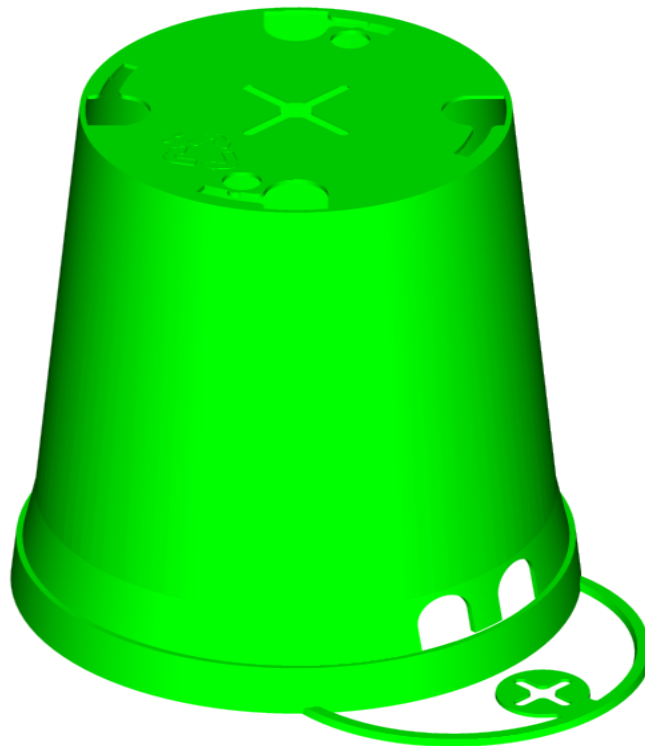
Figure 2. New trap base with modified device for mounting base onto a bamboo stake.
