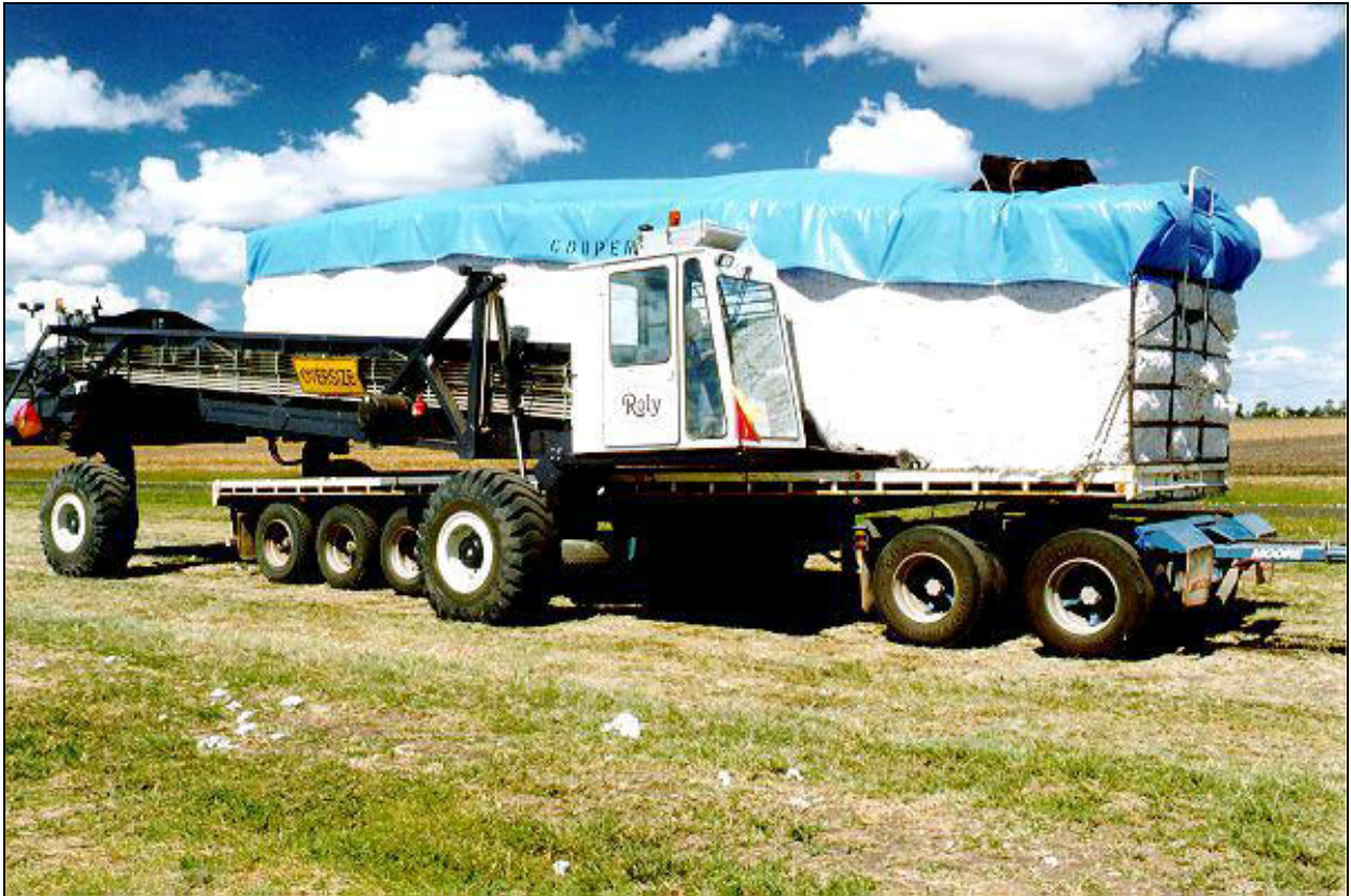
Figure 4: Module loader system used in Australia. Provided by © The State of Queensland Department of Natural Resources 2000.
