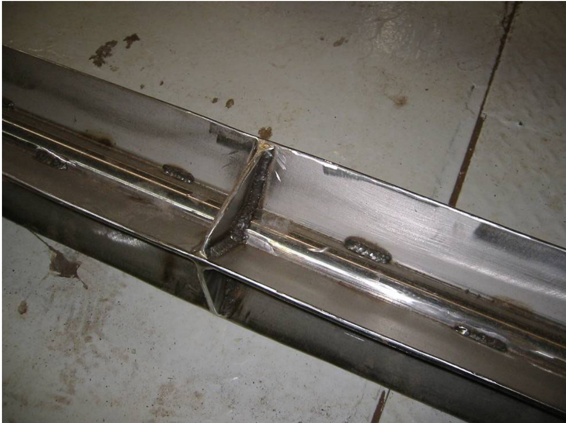
Figure 5. Gussets added to Power Roll gin stand power rolls.
