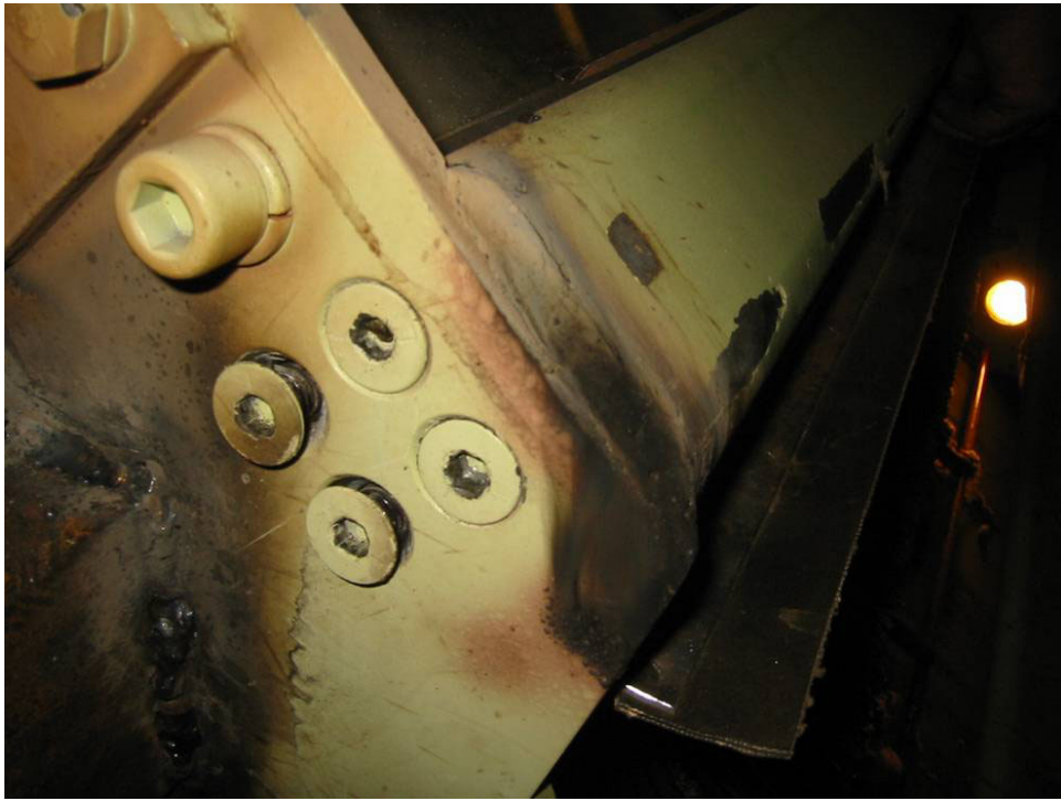
Figure 4. Welded Power Roll gin stand rib rail.
