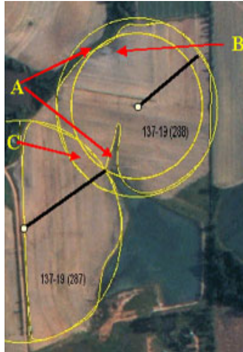
Figure 1: The new tools better place water where, when needed and at the exact needed rate. Off target water applications like roads, waterways and non-cropped areas (A), boggy spots (B), or overlapping pivot areas (C), as shown in this aerial photo are reduced or eliminated.
