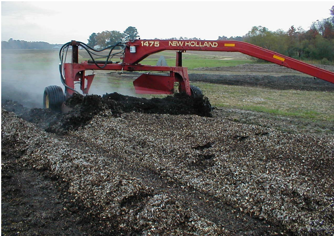
Figure 2. Windrow turner shown turning windrow after 30 days of composting.
