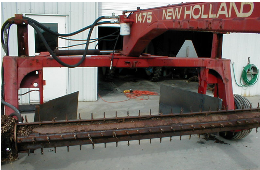
Figure 1. Windrow turner built by replacing the disc cutters on a swing-tongue mower-conditioner with a spiked roller. (Frame donated to the project by CNH, New Holland, PA and modified by Commonwealth Gin, Windsor, VA.)
