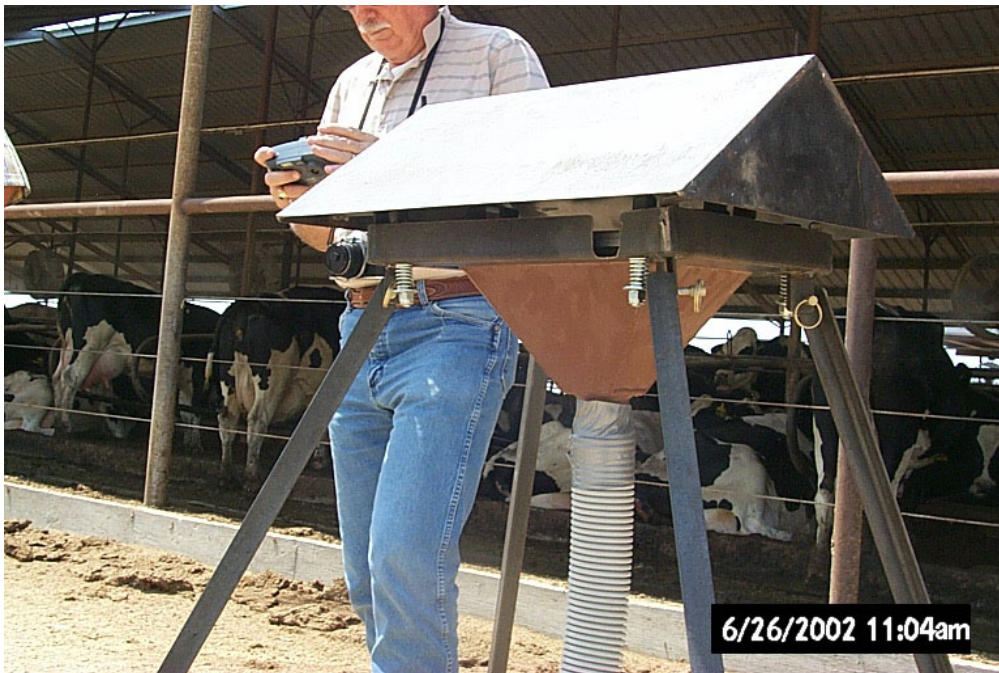
Figure 3. Machinery detent pins are integrated into sampler to allow the legs to be removed thus reducing storage space required.
