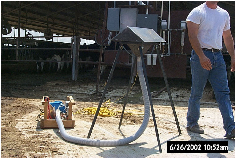
Figure 2. TAMU HiVol TSP sampler has wider base and more stable footing.
