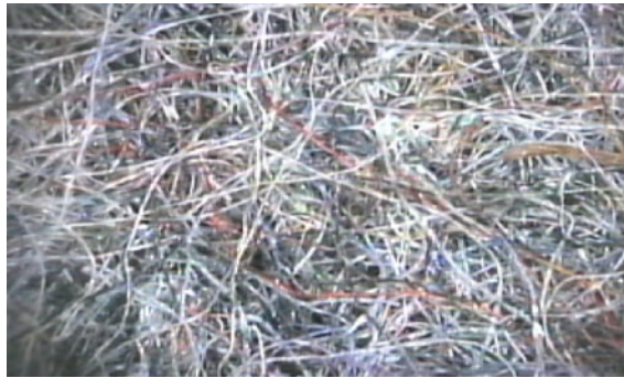
Figure 23. Surface (left) and cross section (right) of a cotton-epoxy composite, sample thickness 5 mm, magnification 100 x.s.
