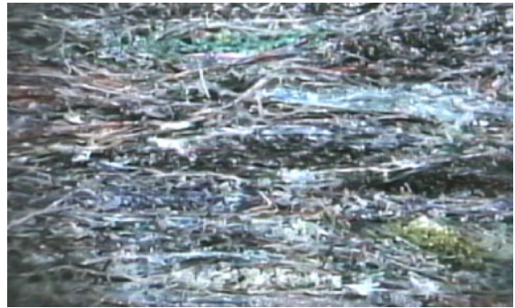
Figure 23. Surface (left) and cross section (right) of a cotton-epoxy composite, sample thickness 5 mm, magnification 100 x.s.
