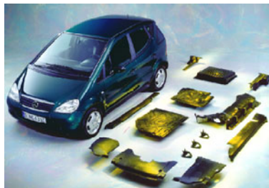
Figure 14. Concepts of pre-serial products for exterior automotive parts made of natural fiber reinforced composites [17].
