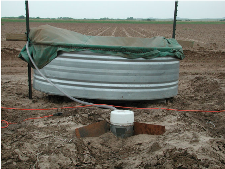
Figure 1. Runoff collection system. Runoff is channeled into a sunken tube from approximately 50 feet of row and pumped into a 6-foot diameter stock tank.
