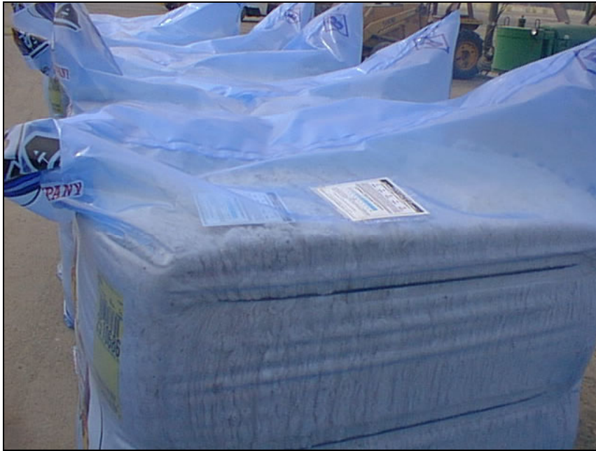
Figure 3. Relative humidity monitor on the outside of the bale bagging.
