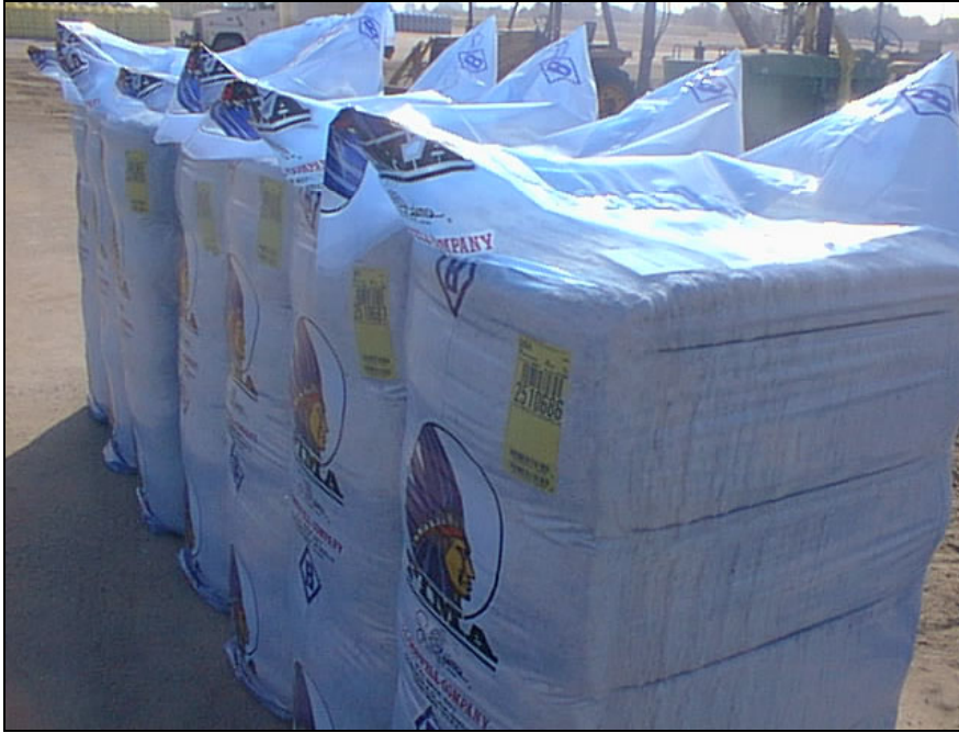
Figure 1. LLDPE film packaged UD cotton bales selected for testing.
