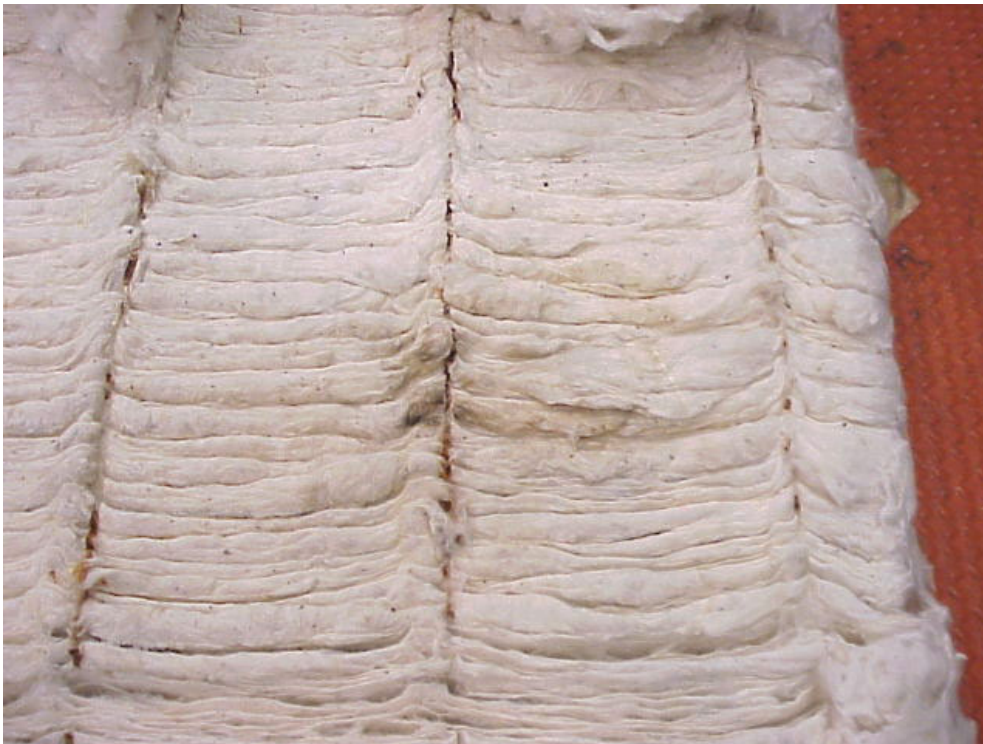
Figure 6. Discoloration occurred at the bale tie for the bales where moisture was added.
