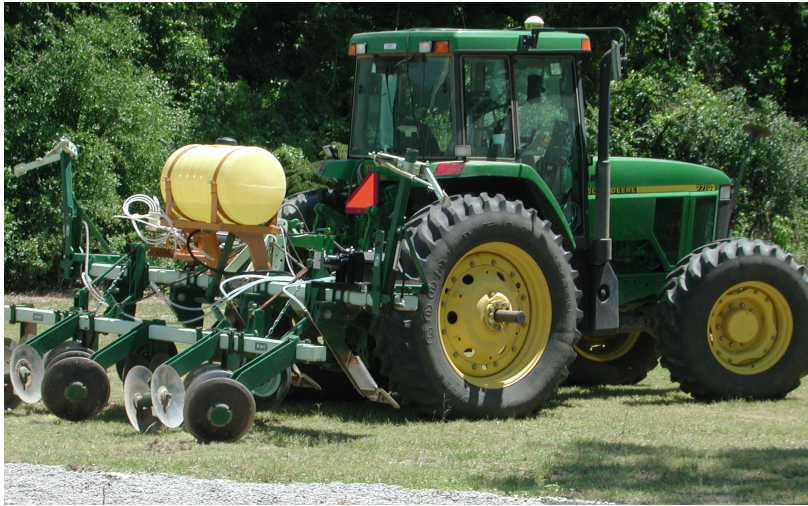
Figure 1. Geo-referenced variable-rate Telone II applicator.
