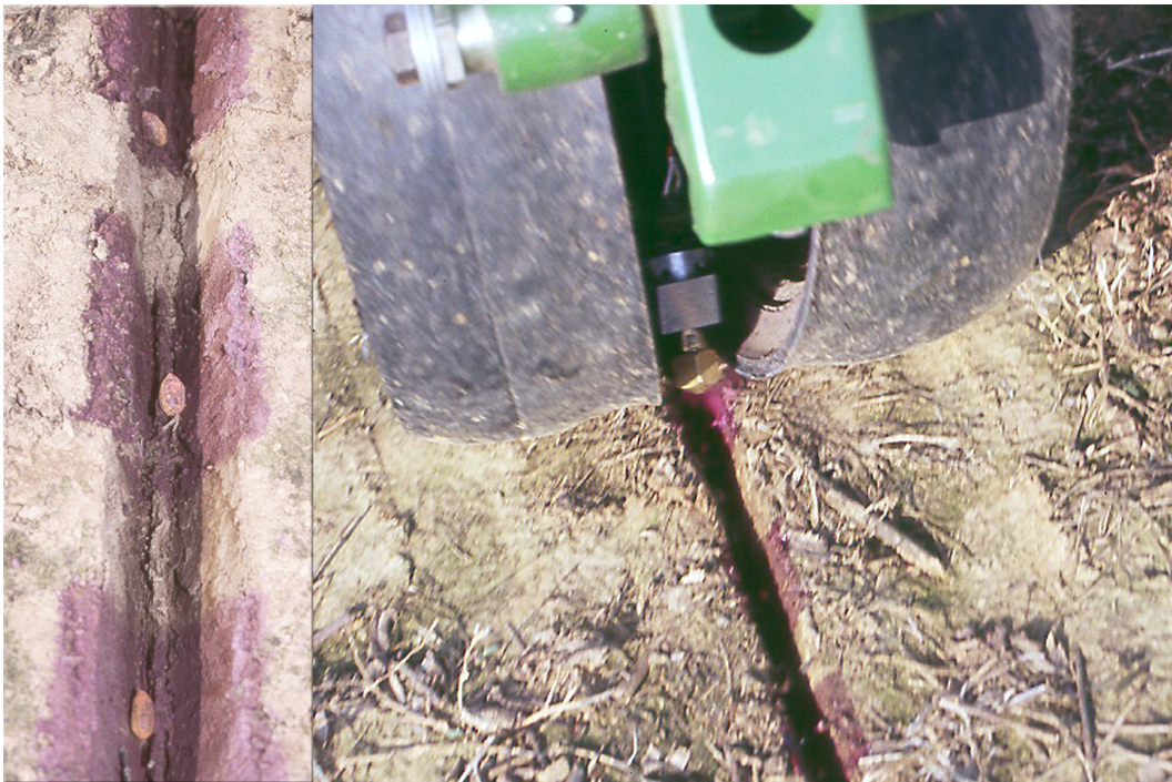
Figure 6. Photos of seed-specific applicator spraying a seed and a furrow closeup.
