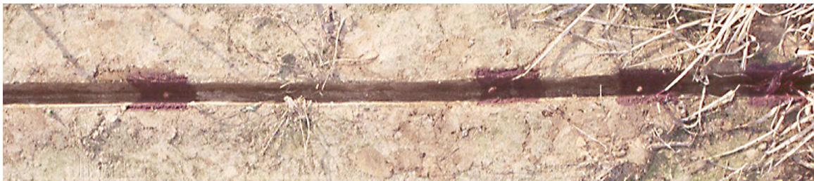
Figure 4. When the seed meter failed to deliver a seed (notice skip in photo), no spray was delivered.
