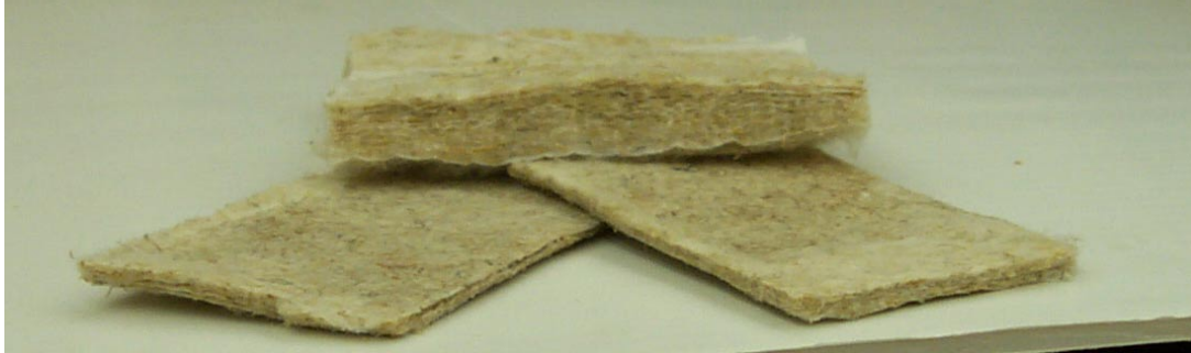
Figure 1. Layered composite nonwovens made of bagasse/cotton webs and Eastar Bio Copolymer melt blown nonwovens before (top) and after hot-pressing (bottom).
