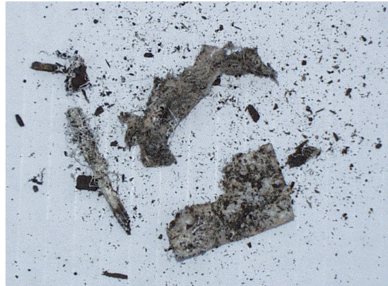
Figure 12. Sample Residual after Burying for 23 days.
