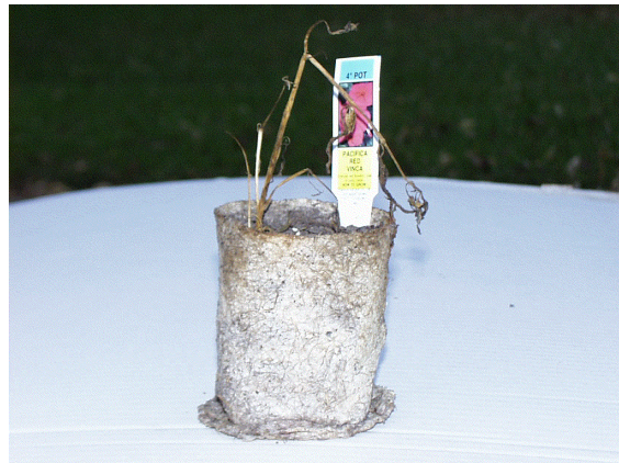
Figure 10. Nonwoven Pot after 100 Days.
