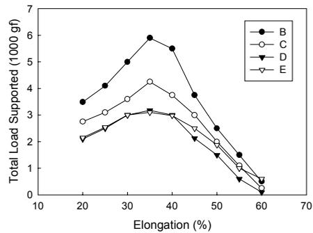
Figure 7. Comparison of the predicted and actual load-elongation curves of oriented web of rayon (1.5", 3.0 denier) for the gage length of 0.75".
