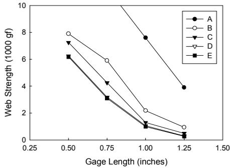
Figure 6. Comparison of the predicted and the actual values of breaking strength of oriented web of rayon (1.5", 3.0 denier).
