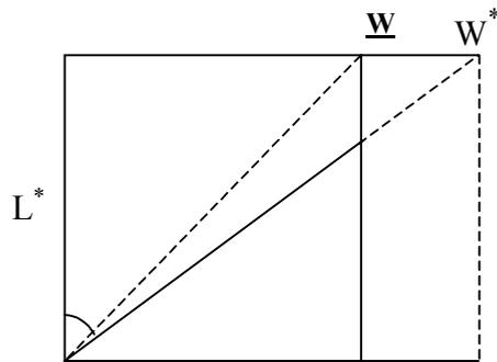
Figure 3. A model of unoriented web between jaws.
