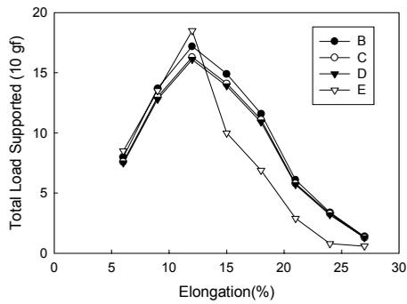
Figure 9. Comparison of the predicted and actual load-elongation curves of unoriented web of rayon (1.5", 3.0 denier) for the gage length of 0.75".
