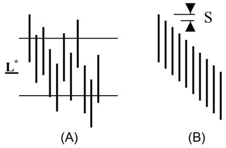
Figure 1. A model of oriented web between jaws. (A) Actual position of fibers, (B) Position after rearranging in descending order of upper ends.
