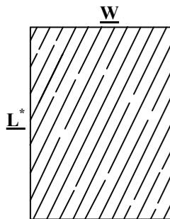
Figure 4. Hypothetical arrangement of fibers in one of the many superimposed layers of a randomly oriented web.
