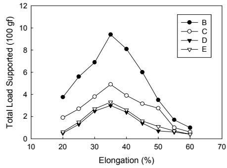
Figure 8. Comparison of the predicted and actual load-elongation curves of oriented web of rayon (1.5", 3.0 denier) for the gage length of 1.25".
