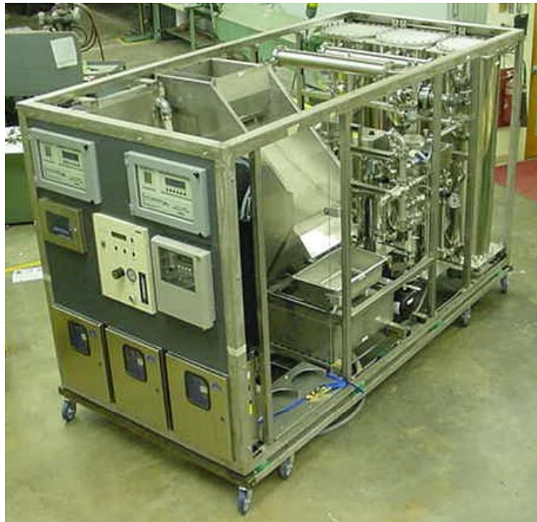
Figure 4. Skid-mounted prototype for UV-enhanced ozonation of wastewaters.
