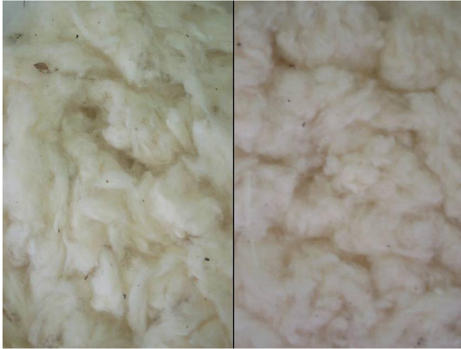
Figure 5. Cotton from bale (left) and from Crosfeed (right) after processing (Bale A).
