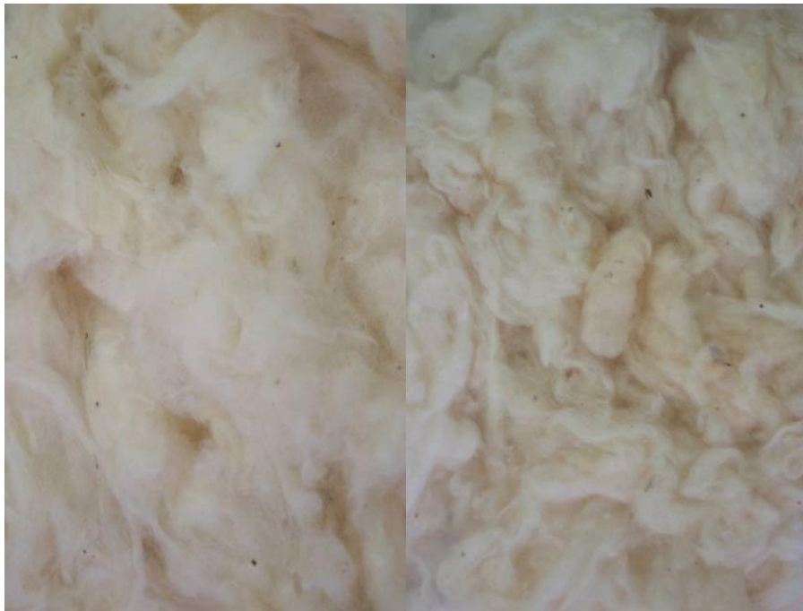
Figure 6. Cotton from bale (left) and from Crosfeed (right) after processing (Bale B).
