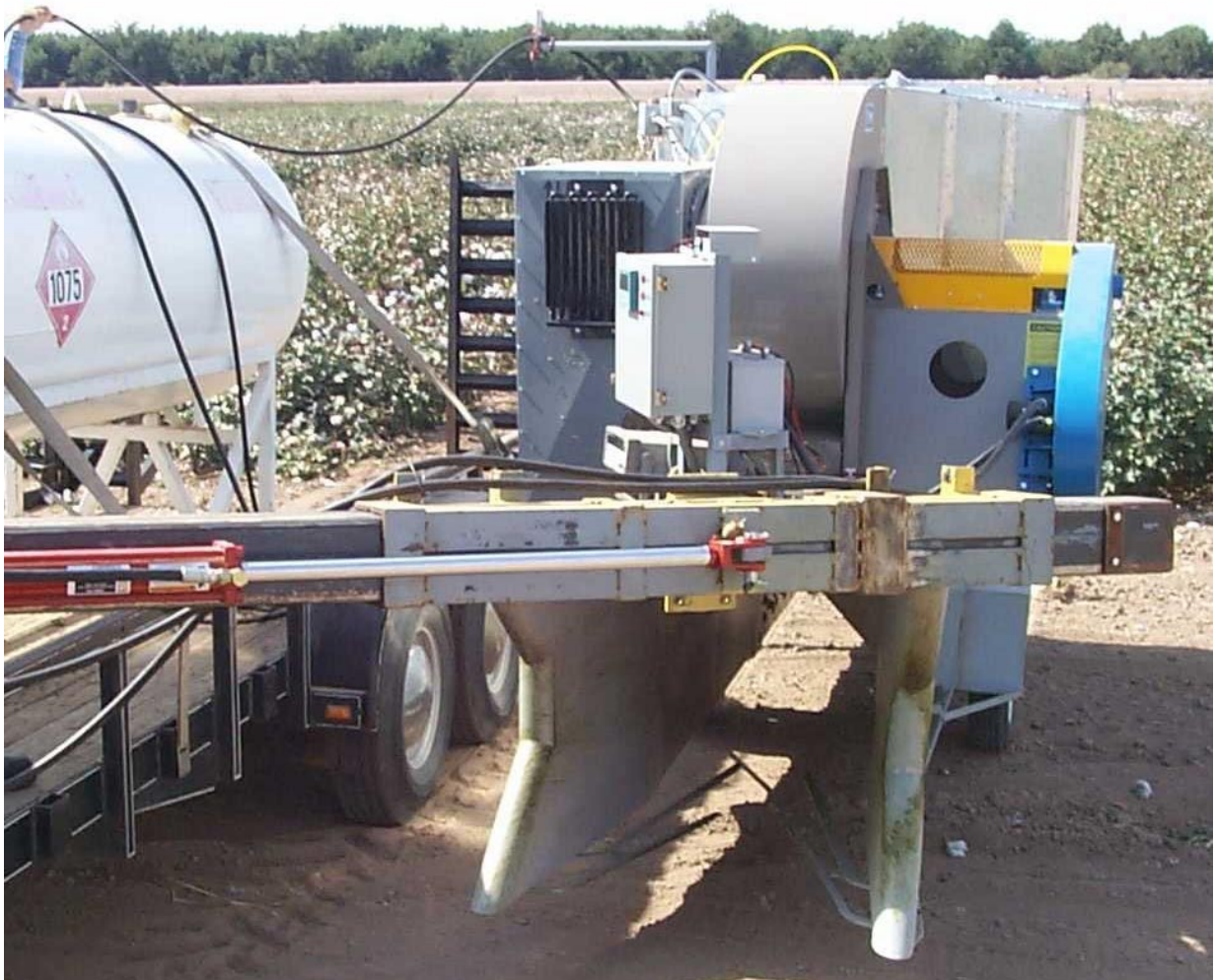
Figure 1. Apparatus built to apply hot air to the cotton canopy. The hydraulic cylinder (on tractor toolbar) positions the device over the inner or outer row.
