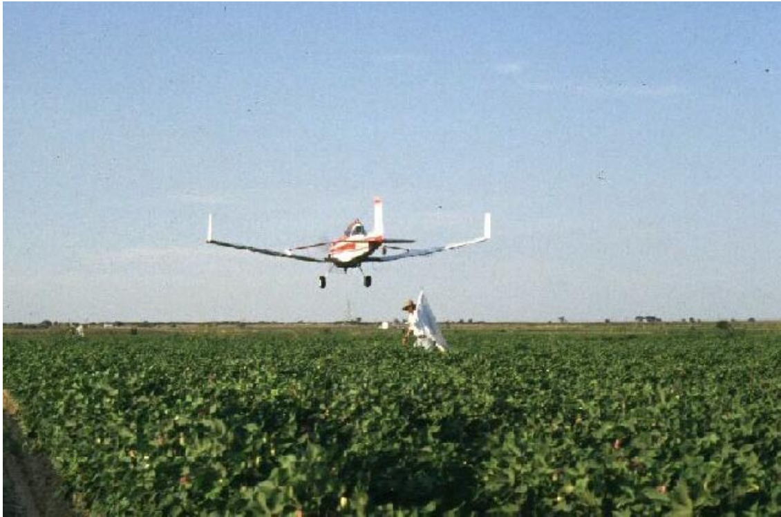
Figure 1. Cessna Ag Truck equipped with winglets used in aerial applications of selected formulations of malathion.
