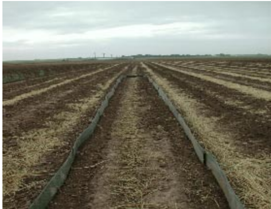
Figure 1. Runoff collection system. Runoff is channeled into a sunken tube (upper left) from approximately 50 feet of row (lower left). Runoff water is pumped into a 6-foot diameter stock tank (upper right and lower right).
