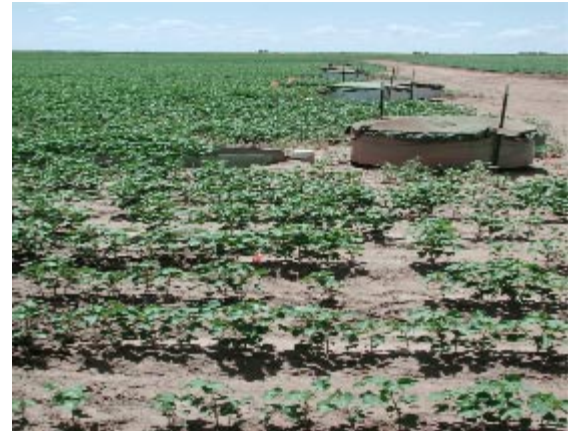
Figure 1. Runoff collection system. Runoff is channeled into a sunken tube (upper left) from approximately 50 feet of row (lower left). Runoff water is pumped into a 6-foot diameter stock tank (upper right and lower right).
