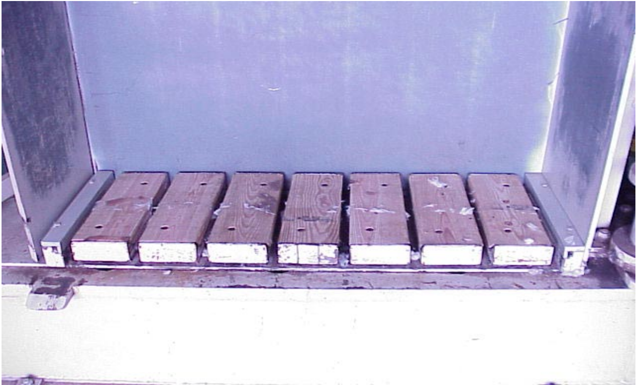
Figure 2. Wooden inserts installed on the shaped platen to make it flat.
