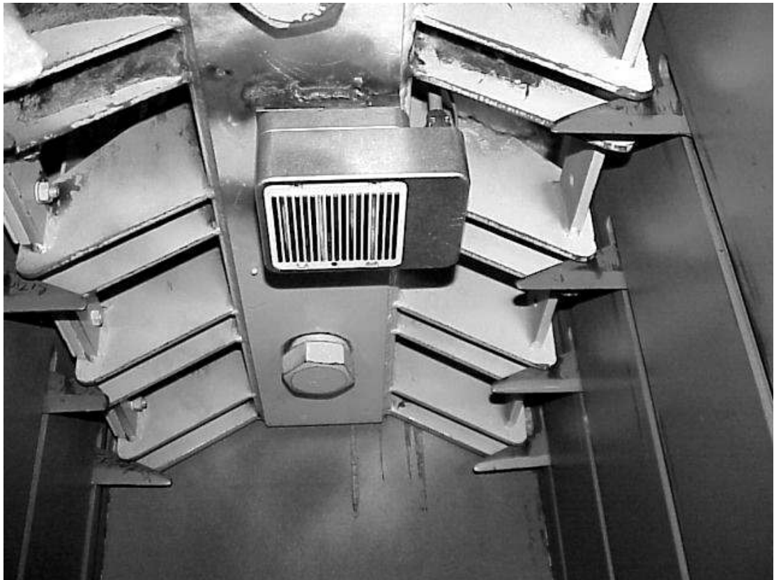
Figure 5. Photograph of tramper located in the bale press showing the moisture-sensing grid.
