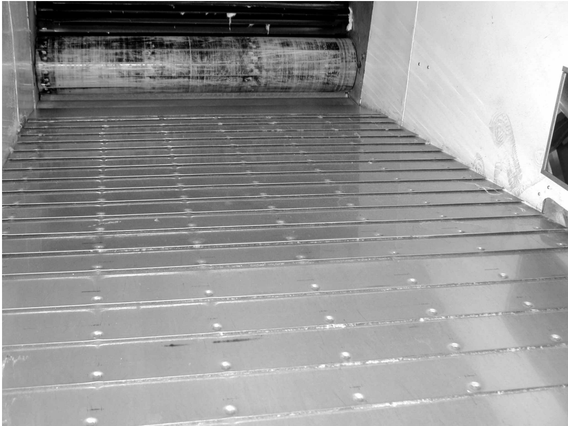
Figure 2. Lint slide grid used in moisture restoration system.
