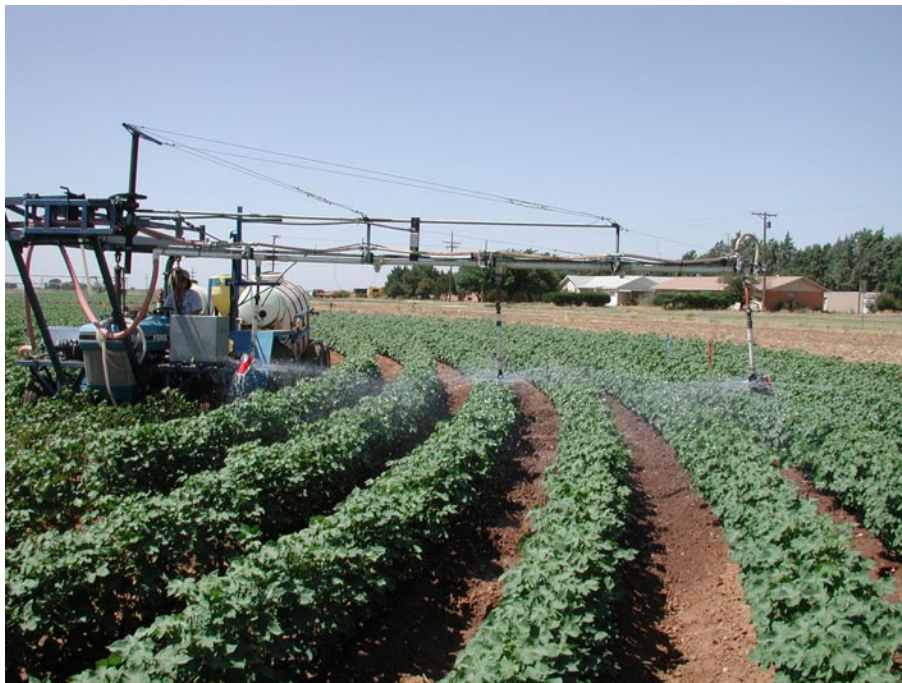
Figure 1. The pivot simulator used to administer treatments of water through three irrigation applicators.
