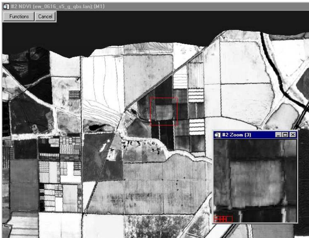
Figure 13a. Image of the normalized difference vegetation index (NDVI) for field 4 obtained from low-flying aircraft and processed using ENVI 3.4. Three faint horizontal lines can be seen in the image.
