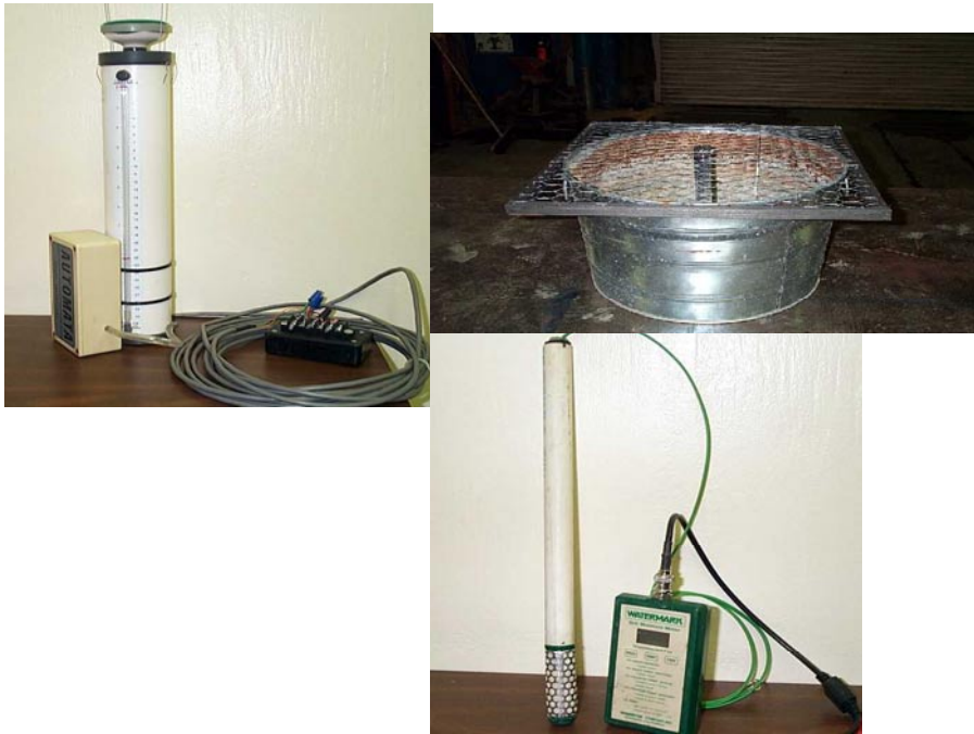
Figure 1. Atmometer evaporation device (top left), washtub evaporation pan (top right), and Watermark 200SS soil water sensor with 30KTCD-NL meter.
