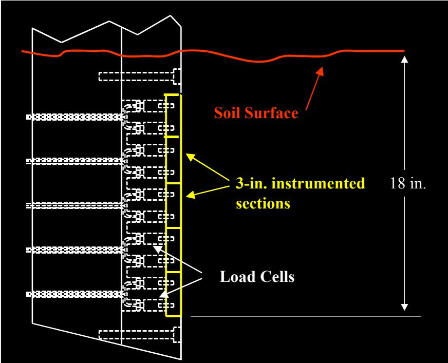
Figure 1. Schematic diagram of the instrumented shank.
