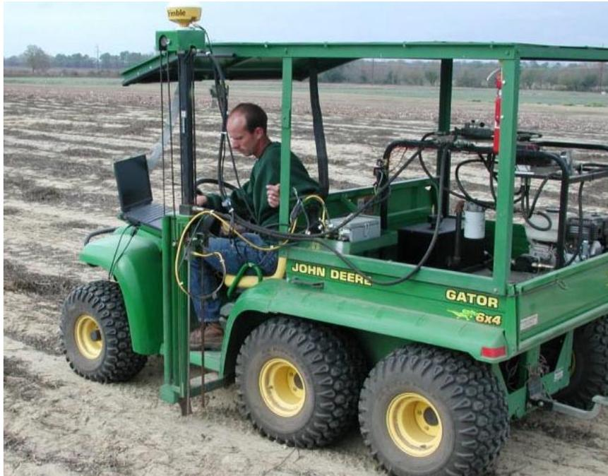
Figure 2. Hydraulically operated, penetrometer system with DGPS unit.
