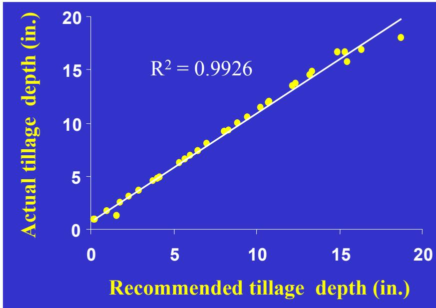
Figure 6. Correlation between recommended tillage depth (from site-specific tillage map) and actual tillage depth performed by the depth-controller system.
