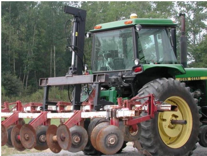
Figure 3. The control system for variable-depth tillage operations.
