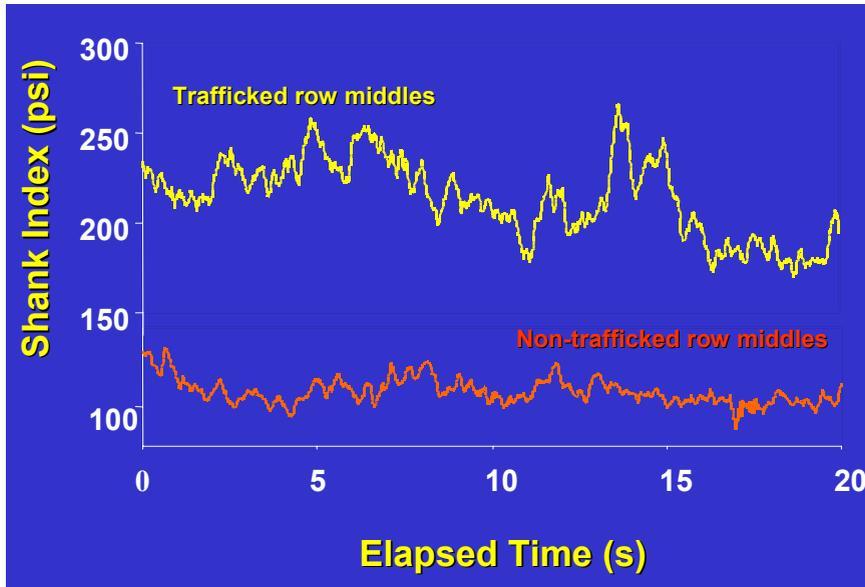
Figure 4. Shank index data from trafficked and non-trafficked row-middles for the 3-in. section operating 9 to 12 in. deep.
