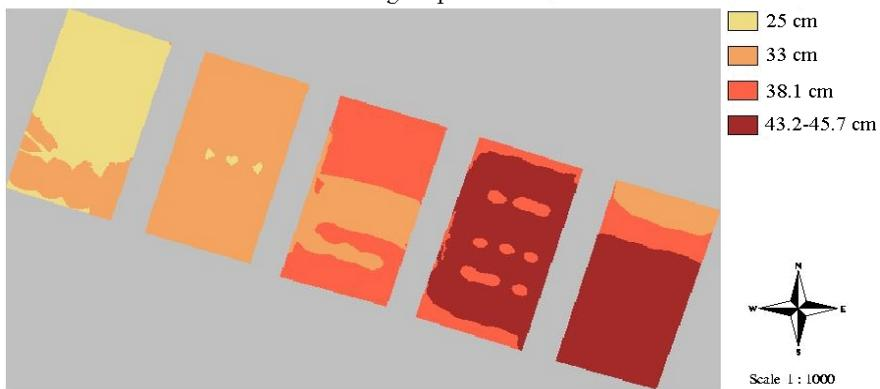
Figure 7. Predicted tillage depths necessary to eliminate root-restricting layer for the test field based on soil penetrometer data.
