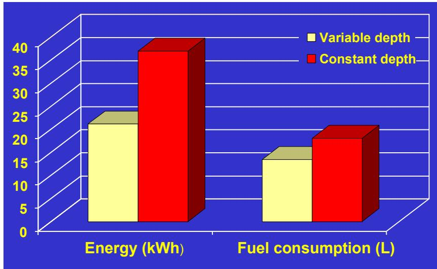
Figure 9. Energy and fuel requirements of constant and variable-depth tillage systems.
