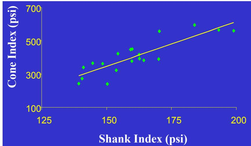
Figure 5. Correlation between soil strength values average over 9 to 12 in. depths as measured with the con penetrometer (cone index) and the instrumented shank (shank index).
