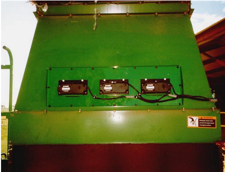
Figure 3. Emitters mounted on the outside (basket side) of the cleaner.
