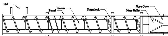
Figure 1. Extruder Barrel Cross-Section.
