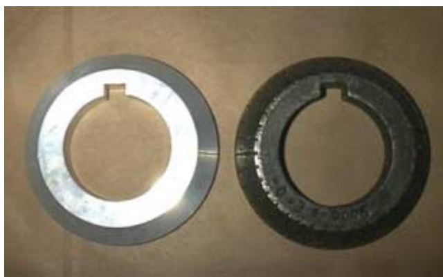
Figure 4. Aluminum wear disk used for test (left) versus conventional cast iron steam lock used in the extruder (right).
