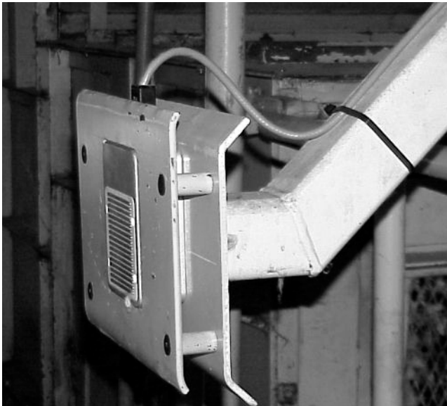
Figure 5. Bale pusher with moisture sensor at Burdette Gin.
