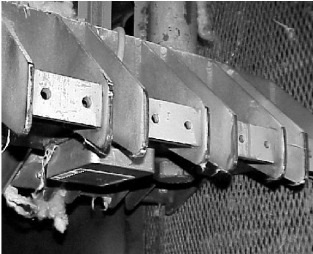
Figure 4. Lint moisture sensor attached to tramper at McClendon, Mann, and Felton Gin.
