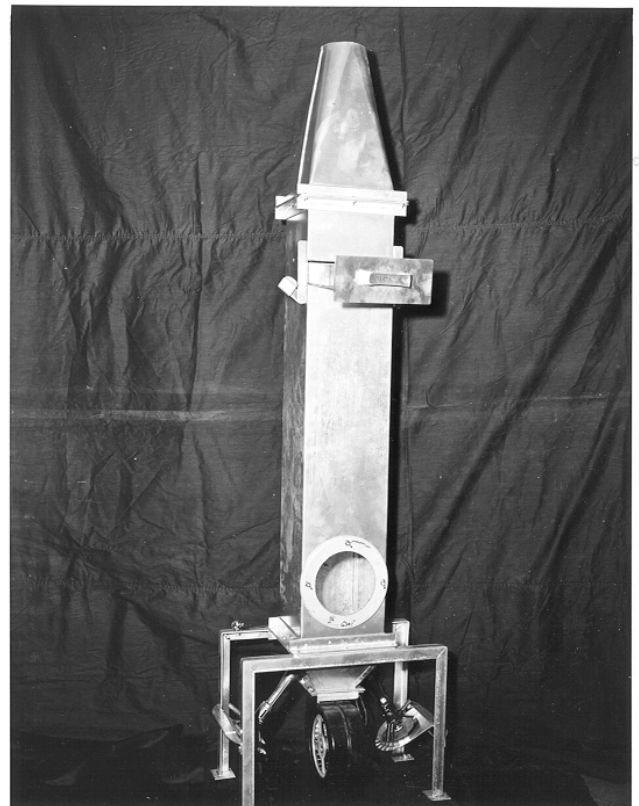
Figure 8. Laboratory constructed drier for close control of temperature and exposure period (67-42-85).
