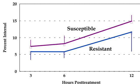
Figure 1. Penetration of [<sup>14</sup>C]spinosyn A through the dorsal cuticle of last stadium tobacco budworms. Data are the means of 5 larvae; dispersion bars are 1 standard deviation.
