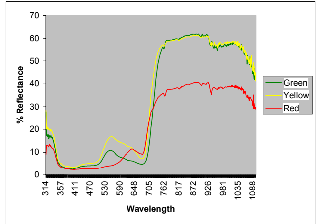
Figure 3. Reflectance spectra for cotton leaf types in mite infested fields, Stoneville, MS, 8/11/00.
