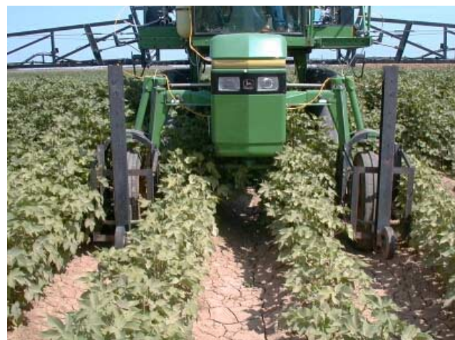
Figure 1. Optical height sensor mounted in front of high-clearance sprayer
