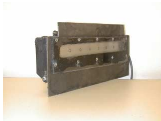
Figure 1. Modified MicroTrak cotton sensor. Both emitter and detector units had the same design.
