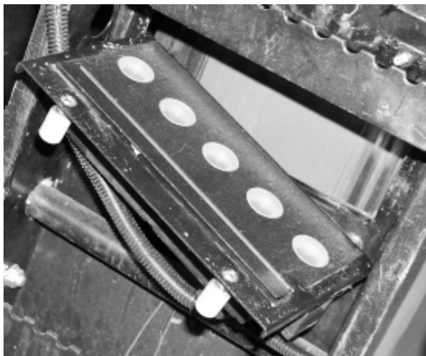
Figure 2. AgLeader sensor detached from duct.
