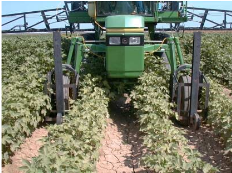
Figure 3. Optical height sensor mounted in front of high-clearance sprayer.
