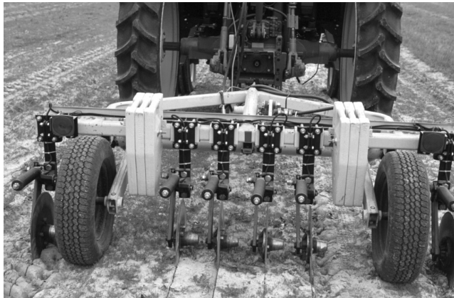
Figure 1. Veris Model 3100 Electrical Conductivity Mapping System.
