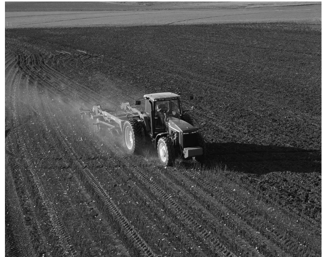
Figure 2. Working in standing stalks, the 2700 mulch ripper has the ability to leave a "smooth and level" soil profile. The right side of the tractor shows the smooth soil profile produced by the 2700.
