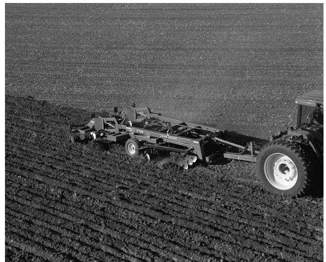
Figure 3. Working after stalks have been shredded, the 2700 mulch ripper has the ability to leave a "rougher" soil profile to meet Highly Erodible Land (HEL) requirements.
