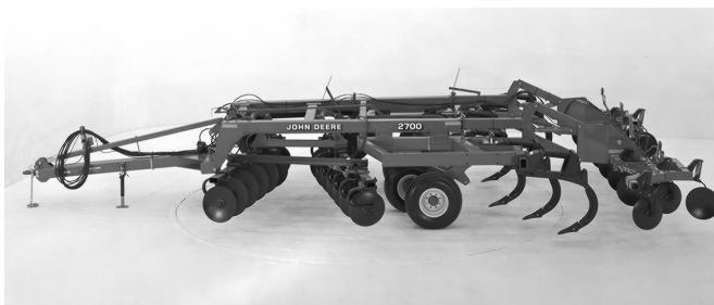
Figure 1. The 2700 mulch ripper configuration from fore-to-aft of the tool consists of the following: disk-disk-ripper-conditioner.
