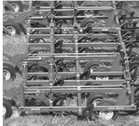
Figure 3. AccuDepth controls the primary and intermediate depths and side-to-side leveling from the operator's seat.
