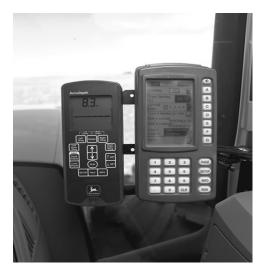
Figure 1. The AccuDepth control system is designed to meet customers' needs for precise and accurate tillage. Illustrated in this picture are the two displays for the AccuDepth control system—the AccuDepth display on the left and the GreenStar<sup>TM</sup> display on the right.
