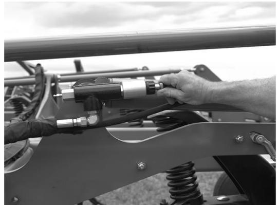
Figure 4. Sensors at the wheels work with a controller and cab-mounted console. As the operator makes adjustments, cylinders at each wheel have a proportional valve and potentiometer that react, raising and lowering each section separately.
