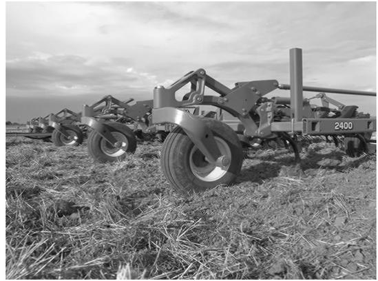
Figure 2. The floating hitch on the 2400 chisel plow offers uniform consistency of tillage depth from front-to-back and side-to-side.
