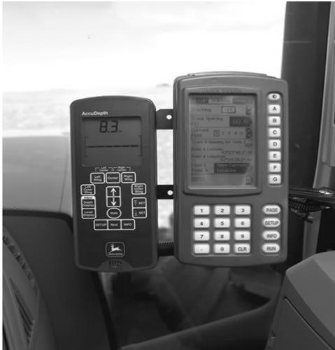
Figure 1. The AccuDepth control system is designed to meet customers' needs for precise and accurate tillage. Illustrated in this picture are the two displays for the AccuDepth control system—the AccuDepth display on the left and the GreenStar™ display on the right.
