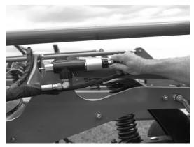
Figure 4. Sensors at the wheels work with a controller and cab-mounted console. As the operator makes adjustments, cylinders at each wheel have a proportional valve and potentiometer that react, raising and lowering each section separately.
