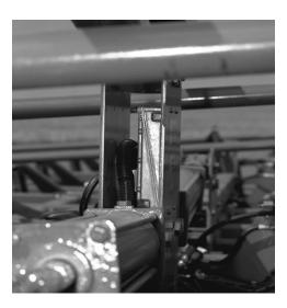
Figure 5. The controller stores set points, sends signals to the proportional valve, receives height sensor signal, and communicates the position to the display. It is located between the wing towers on the center frame of the implement.
