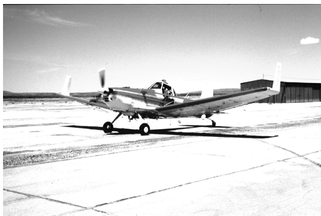
Figure 1. Cessna Ag Truck with winglets used in aerial applications of malathion.
