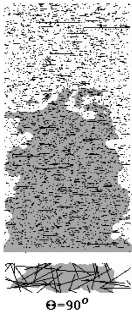
Figure 13. Vertical and horizontal cross – section of textile sample model after 600 MCS. Horizontal cross – section belongs to the high 150 l.u. Fibres of the sample are parallel with the original liquid surface ( \theta = 90^\circ ).
