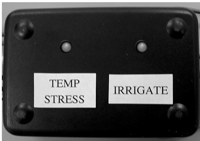
Figure 1. The in-field display of the BIOTIC as implemented in 1998 field study. The two LEDs indicate the thermal status of the crop. The thermal stress LED is lighted whenever the temperature of the canopy is in excess of the temperature threshold. The irrigation LED is lighted whenever the 5.5
