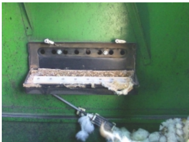
Figure 1. Sensor module mounted inside field cleaner. Module is opened for cleaning.
