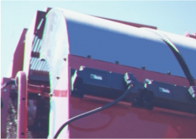
Figure 2. Two emitter units mounted on the front of a double-width chute on a Case IH cotton picker.
