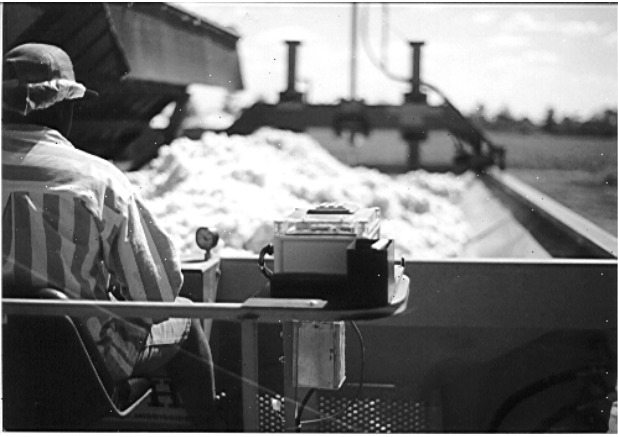
Figure 2. The display and data logger were located in box in center of the figure on the module builder.
