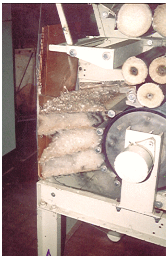
Figure 1. Sheet metal deflectors used to capture trash from each grid bar of a 16-D lint cleaner.
