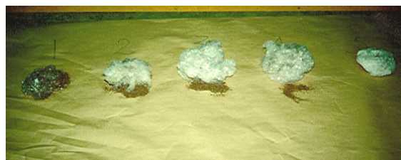
Figure 2. Samples of waste from each grid bar of a 16-D lint cleaner are shown with grid bars from 1 to 5 presented left to right. The four samples on the right were cleaned with a Shirley Analyser and the relative amounts of fiber and plant parts are shown.
